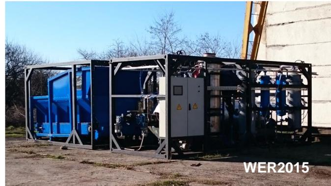
The WER turns waste into gas which could be used immediately after being produced. The working process is as follows: the waste is taken in, the WER converts it by high temperature slow pyrolysis into gas with integrated gas cleaning, and the gas is used locally to provide the energy for which there is local demand.
